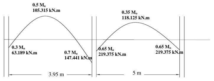
b.Lateral distribution of moment at exterior panel (column and middle strip moments at exterior support) Homework!
